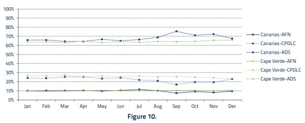
FANS Datalink Air-Ground Traffic Distribution (Uplink and Downlink)
